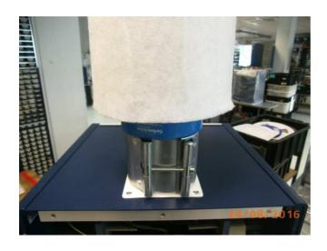
Tighten the screws of the clamping piece until the parts are fixed.
