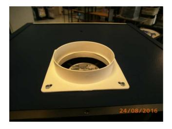
Fix the connection piece on the opening hole on the top of the unit.
