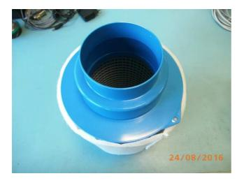
Stick the two parts of the active carbon filter together
