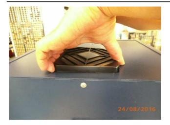
Remove the filter element on the top of the device.
